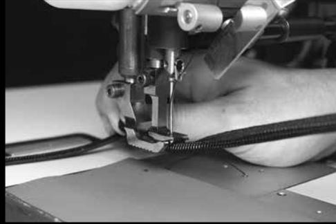
2) Set up chain with sewing foot
